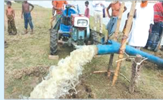
Axial flow pump in operation
